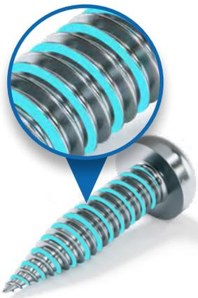
Due to the generated pull-through, the created internal thread is longer than the sheet thickness. In addition the thread pitch of QUICK FLOW® Plus is finer than the pitch of conventional sheet screws, which means that there is sufficient overlap of the formed thread flanks to create a stable joint. The QUICK FLOW® Plus thin sheet screw has a double thread. This additionally increases the surface area of the engaged thread flanks.
